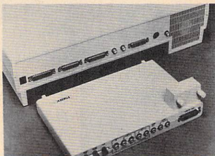
Commodore's Genlock 1300 has plugs for video and audio input and output and connects to the RGB socket of the Amiga.
