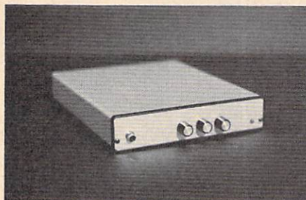
ProGen from Progressive Peripherals merges Amiga and video graphics by replacing color 0 on the Amiga with the video input.
