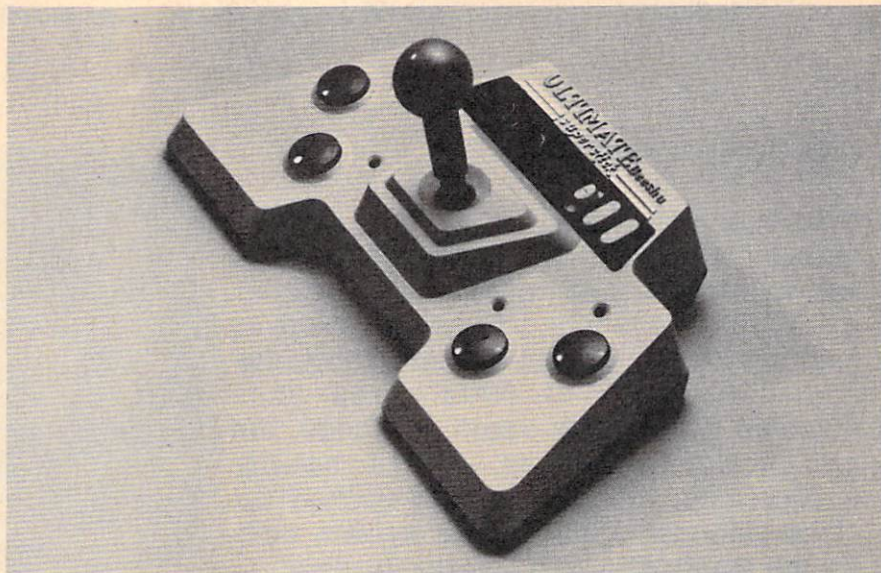
Beeshu's Ultimate Superstick has a ball-style stick with four trigger buttons, two speed controls, and auto-fire controls.
