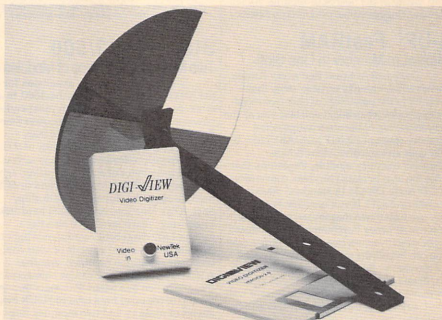
NewTek's Digi-View video digitizing system includes software, an interface, and a color-filter wheel.
